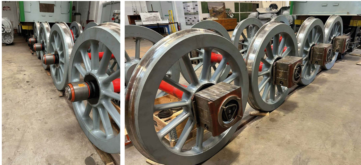
Top and centre: Roller bearings and axleboxes being fitted to the P2 tender wheelsets.
