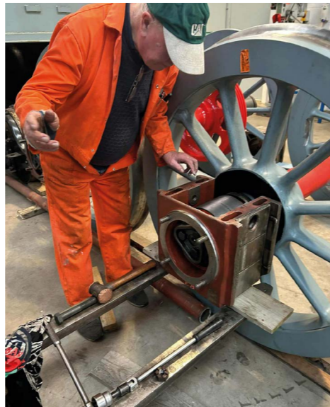
Top and centre: Roller bearings and axleboxes being fitted to the P2 tender wheelsets.
